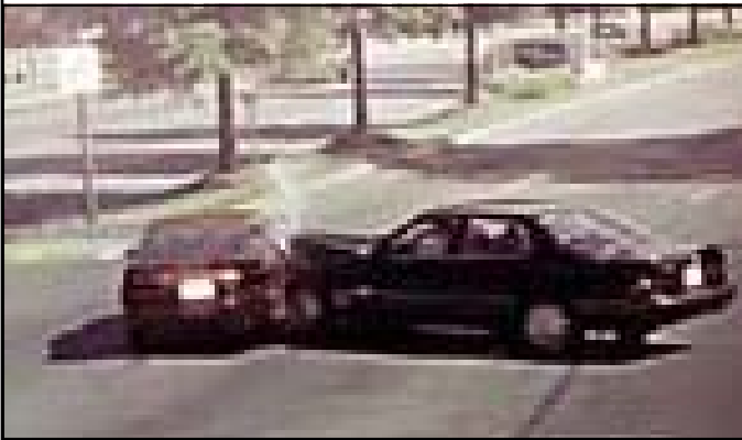
A T-bone crash, the most deadly. Speed at time of this collision: 90 km/hr. Crash severity, and the likelihood of injury or death, increases with speed.
